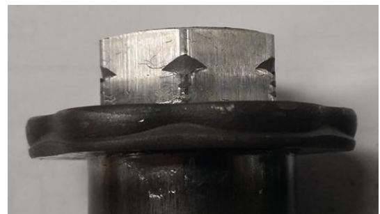
Fig. 3 Damage critical point of 5.5mm at Round 0.3 for Forging Try out TEST
