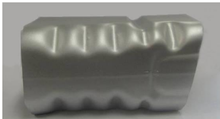
Fig. 11 Hydroformed final shape after cutting
