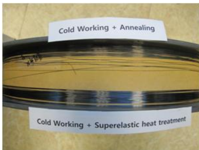
Fig. 6 NiTi wires with a diameter of 0.3mm.
