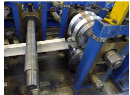
Fig. 5 Roll Forming experiment
