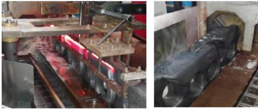
Fig. 2 Induction hardening process using the stop heating
