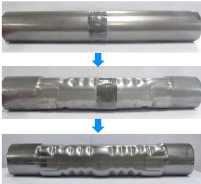
Fig. 10 Hydroforming test process
