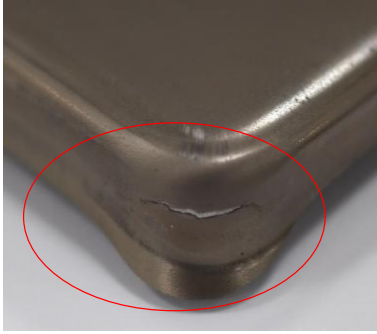
Fig. 1 Experiments of the clad plate forging with torn corner
