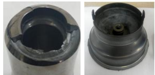
Fig. 1 Crack of Punch and assembly of Engine Mounting Parts
