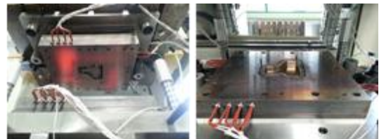
Fig. 1 Die set for HPF of center pillar model
