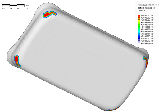
Fig. 5 FLD distribution at the final stroke
