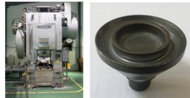
Fig. 5 Final mounting parts of sizing forging
