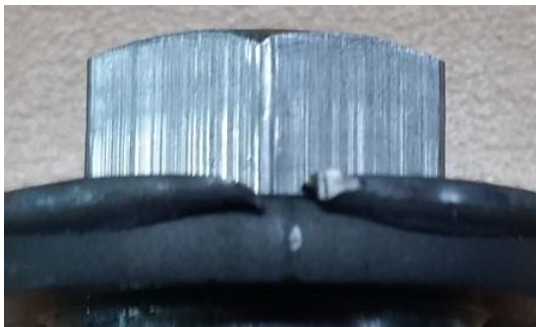
Fig. 5 Damage critical point of 5.5mm at Round 0.8 for Forging Try out TEST
