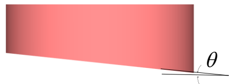
Fig. 2 Initial geometry of workpiece with a tilted end by 5degrees
