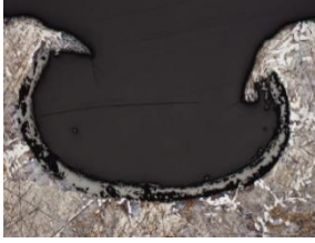
Fig. 2 A typical U-shape pinhole with scale
