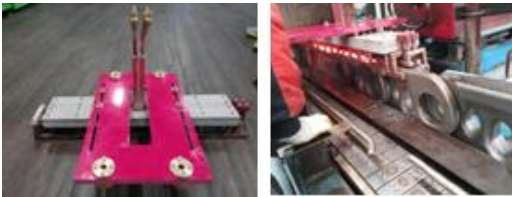
Fig. 4 Induction hardening coil and work process
