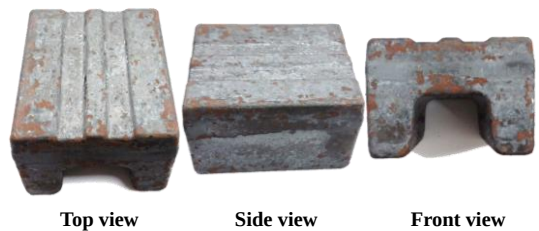
Fig. 9 prototype product by hot forging test
